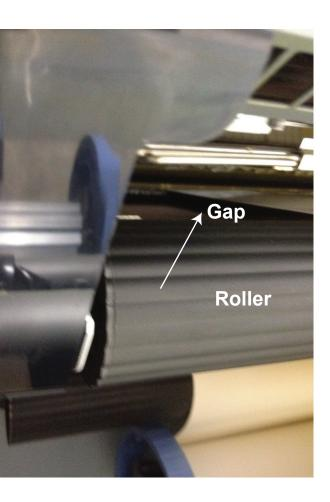
260 - Notice material barely touches out feed and has a roller at the end of the out feed.
