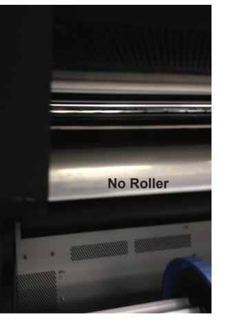
360 - has a longer out feed trey "without" a roller at the end. The material now has more surface contact and when the material has more contact it creates more surface tension that causes the material to bunch up and create a head crash.
