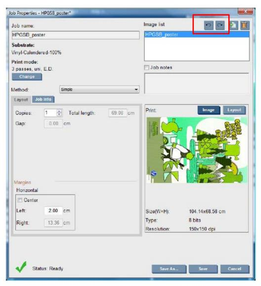
The effect of rotation is shown in the preview. After you press the **Save** or **Save As** button in the Job Properties window, the actual rotation of the job takes place. This could take a few minutes, depending on the image size and resolution, during which the job can be neither printed nor edited, and the job status is shown as Rotating. When it is done, the job is ready for printing.
