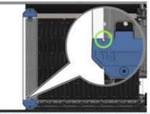
CAUTION: Wrongly positioned edge holders could severely damage the printheads and carriage.
