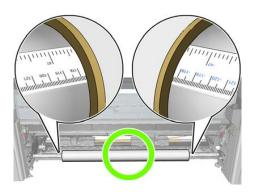
Some lower-quality rolls may be poorly wound onto the cores during manufacturing, resulting in skew and telescoping during printing. This may lead to smears and other image quality issues. The maximum tolerated skew or telescoping according to Latex 3000 printer specifications is 5mm (0.197 in).
