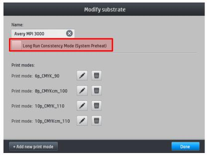
NOTE: The name of this feature for HP Latex 310 and 330 units is just "Long Run Consistency Mode," without the last informative description ("System Preheat").
