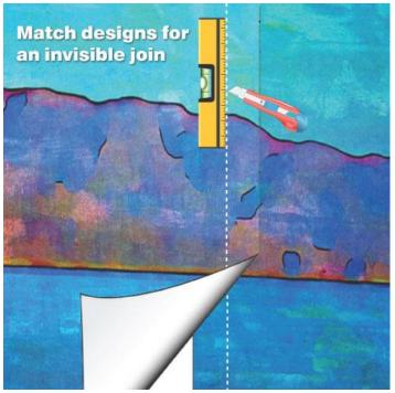
Double Cutting - a technique used to obtain perfectly fitted seams. This is done by overlapping one panel of wallpaper over the other until the image or patterns are perfectly matched. Then a sharp blade is used to cut through both layers. The excess edges are then removed.
