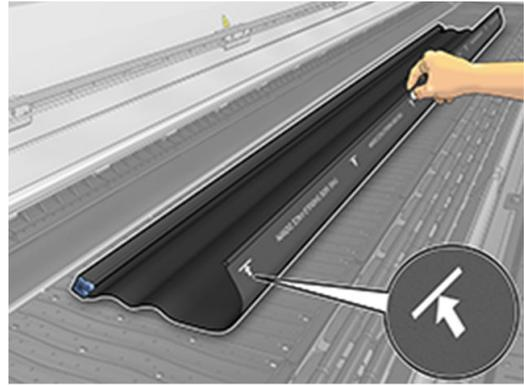
3. To provide the correct tension to the platen protector, place the tensioner element between the platen and the diverter wheels. Make sure the fabric is flat, with no wrinkles.
