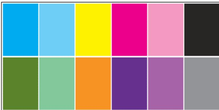
When facing banding issues, print the Image Quality Inspection Plot from the Printer menu: go to Printer > IQ Inspection > Add New Job. This will add a job to the print queue. To print it, edit the details of the job to select the substrate and print mode you want to check. Once the plot has printed, start the troubleshooting process. See the Image Quality Troubleshooting Process image at the end of this section for a summary diagram of the troubleshooting process.
