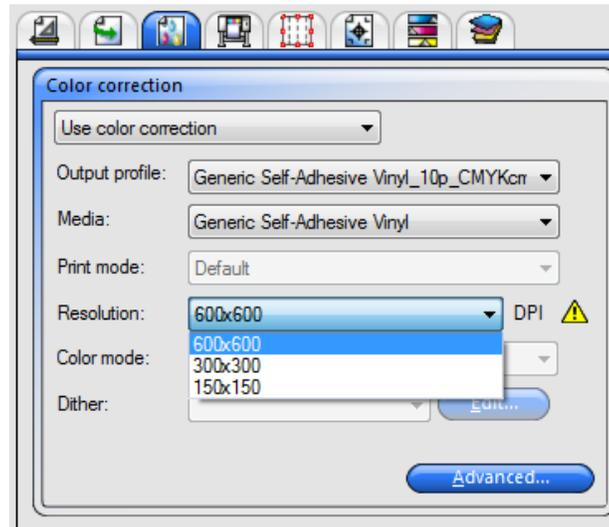
After changing the resolution, a warning message appears next to the selection (“*Your resolution selection does not match what is stored in the ICC Profile*”). This warning message does not prevent printing in the resolution selected. These settings will only apply to the current print job, after which the settings will return to default and the warning message will disappear.
