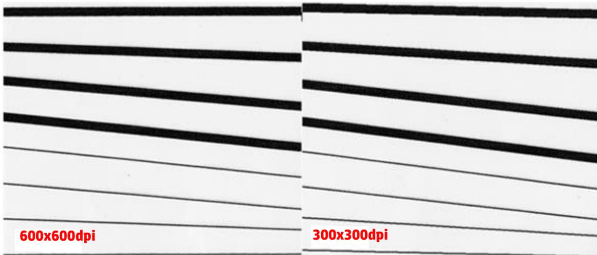
Poor text details have been observed when printing small white letters over a dark background. The most probable cause is insufficient printhead alignment and the advice is to align the printheads using self-adhesive vinyl. If this is not sufficient, then also increase the rendering resolution from 300x300dpi to 600x600dpi from the RIP software. The picture below shows one example of this defect:
