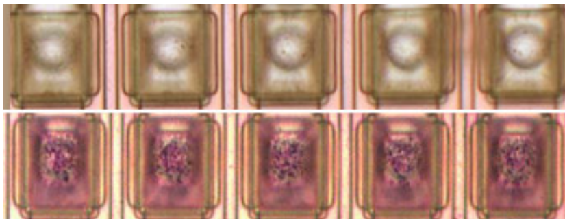
Original HP Latex Inks showing healthy nozzles
