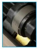
To avoid this, always leave **the pinch rollers in the up position** when the cutter is not in use.
