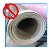
To avoid skew problems when printing and then cutting, please check that the roll of substrate you are going to use does not have any rewinding defects, such as telescoping.
