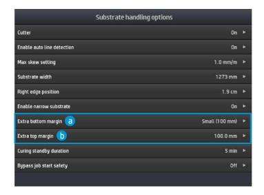
The top and bottom edges of the plot may become wavy; this makes it difficult for the OPOS sensor to read the HP barcode correctly and apply an accurate alignment if insufficient margins are used.
