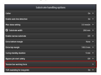
If the **Take-up reel is loaded with the printed side out** (meaning **high tension**) but even **higher front tension** is required, then you should select **Extra tension** in the Front Panel. "High" is the default selection in this configuration.
