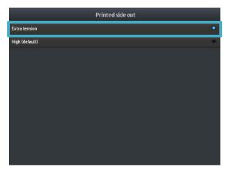
When the Take-up reel is loaded with **printed side out** and the **high tension** setting (default) is selected, it is possible to enable **TUR rewinding for long plots** in the **Substrate handling options** menu. This option modifies the behavior of the dancer bar and improves the rewinding quality. It is recommended to enable this option when printing long runs.
