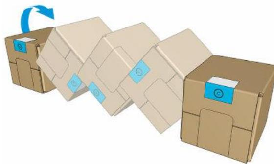
For the White cartridge, shake it 60x times while rotating it to ensure it will be well mixed.
