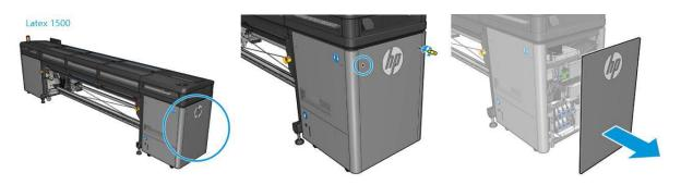
b. Remove the intermediate tank and shake it for 15 seconds before reinstalling.
