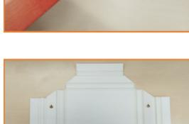
Latex ink flexibility allows 90° bends without cracking the ink. Once the image has been printed, make the necessary V-cuts on the reverse side of the board to create the artwork structure. Also, cut any holes required to hang the artwork.
