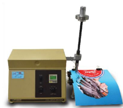
Figure 1. Scratch and abrasion testing are performed using a Taber tester, according to industry-standard test methods.
