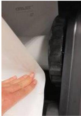
6. Select **Done** on the control panel to lower the pinch wheels again.
