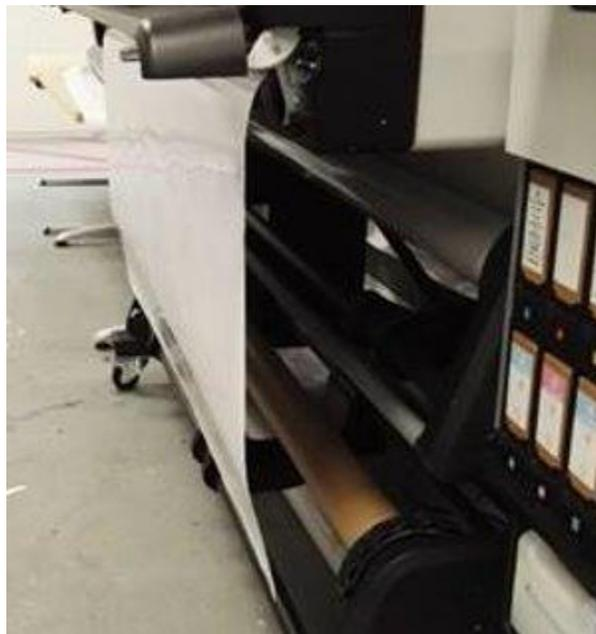
4. Release the pinch wheels: **Substrate** > ... > **Substrate release**.
