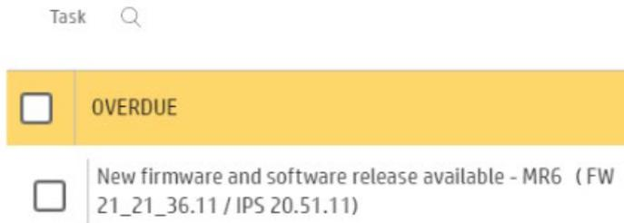
2. By entering maintenance, a list of improvements will be displayed with two buttons, **Install Firmware** and **Install IPS**. Upgrade the firmware first and then the IPS.
