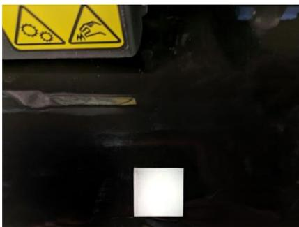
24. The cutter will measure the square and show the calibration values on dx and dy.
