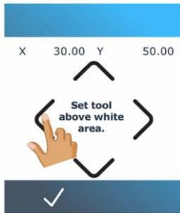
13. The cutter head moves in a circle while measuring the reflection of the substrate.
