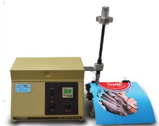
Figure 1. Scratch and abrasion testing are performed using a Taber tester, according to industry-standard test methods.
