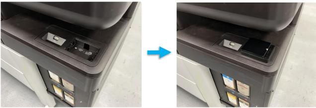
Example of a CAC reader installed in the slot available of selected HP PageWide XL series.
